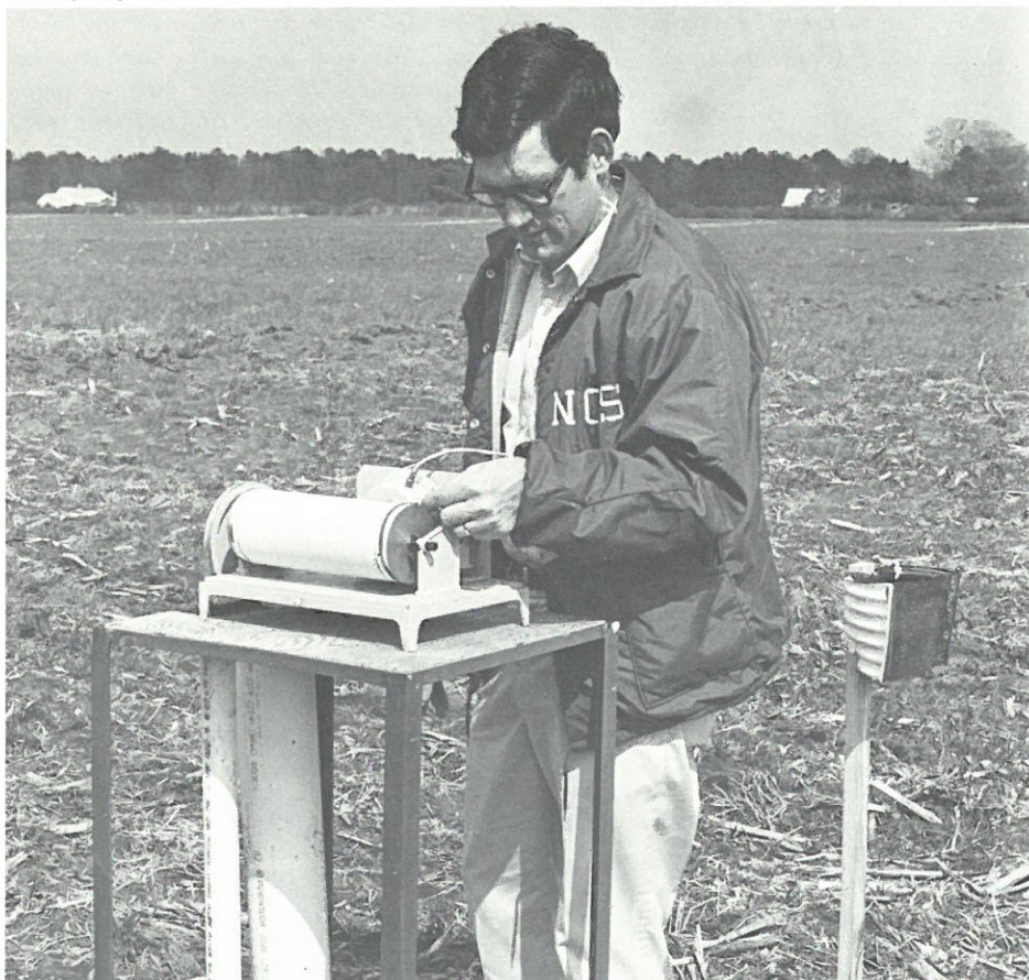
Wayne Skaggs checks equipment which records water table fluctuations
