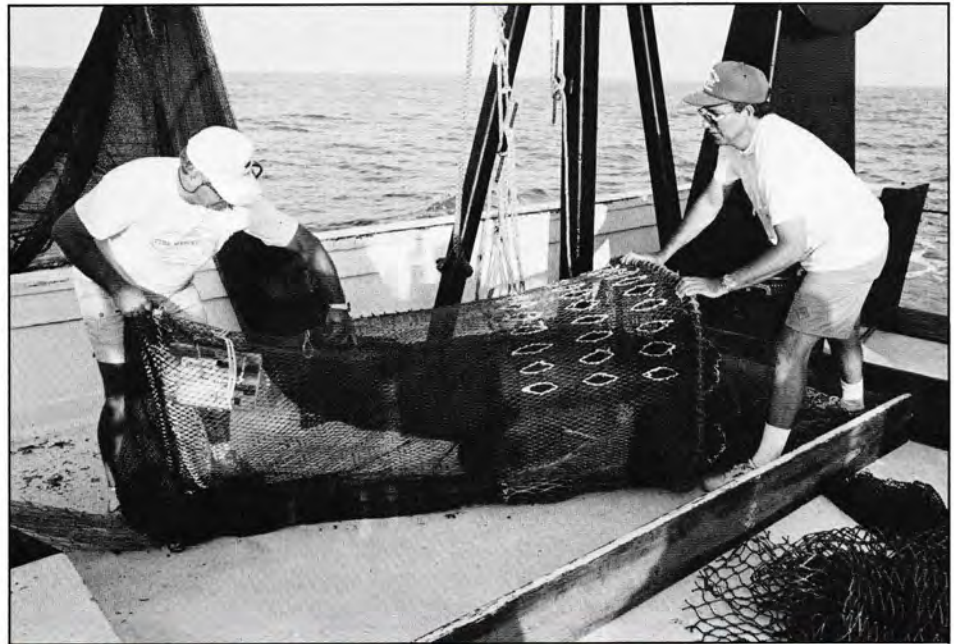
Bahen (left) and Parrish adjust a video camera in the cod end section of the diamond-mesh FSD aboard the Bulldog .
