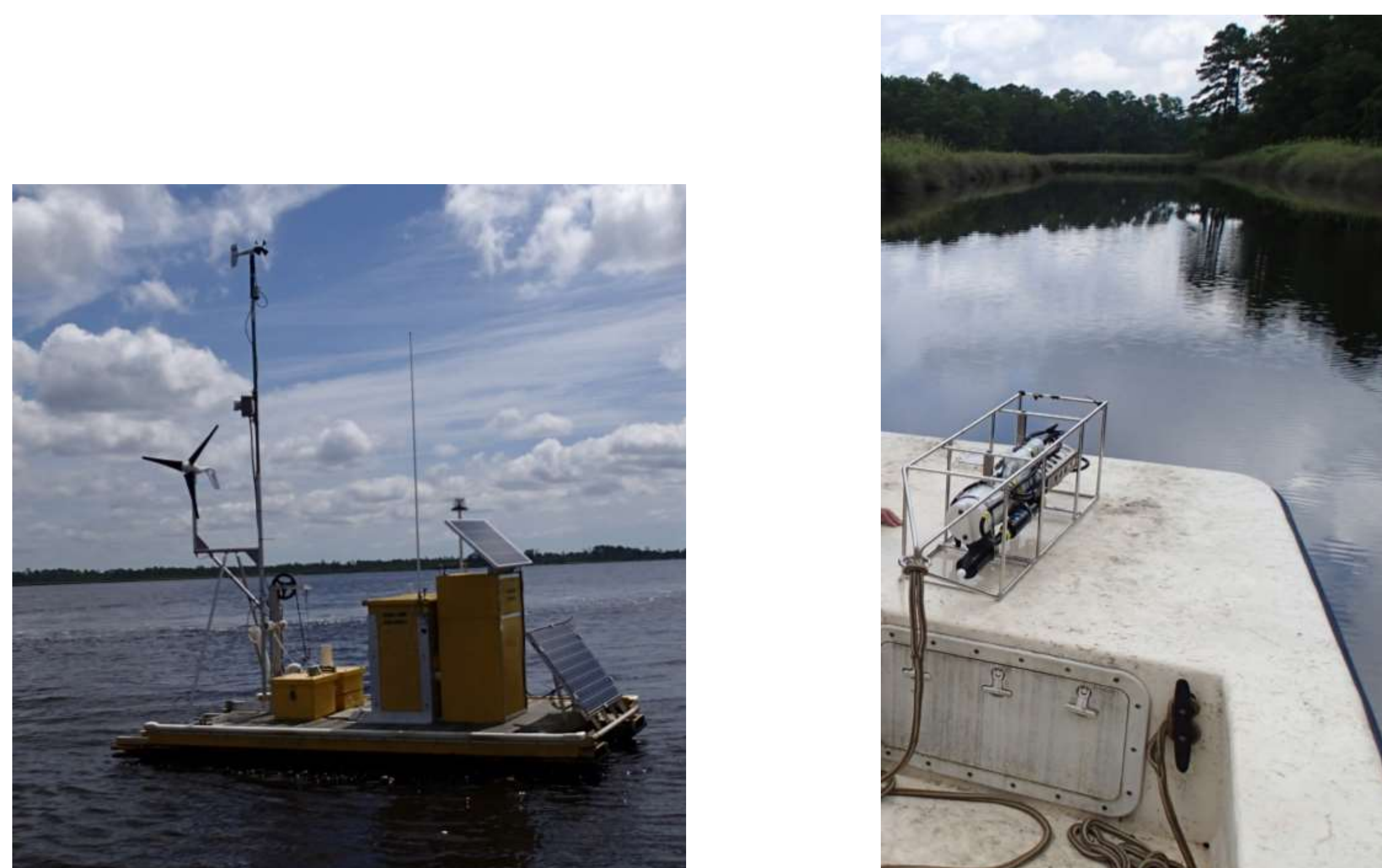
Figure 2. Photographs of (a) the Autonomous Vertical Profiler and (b) the CTD used for the cross-channel transects.
