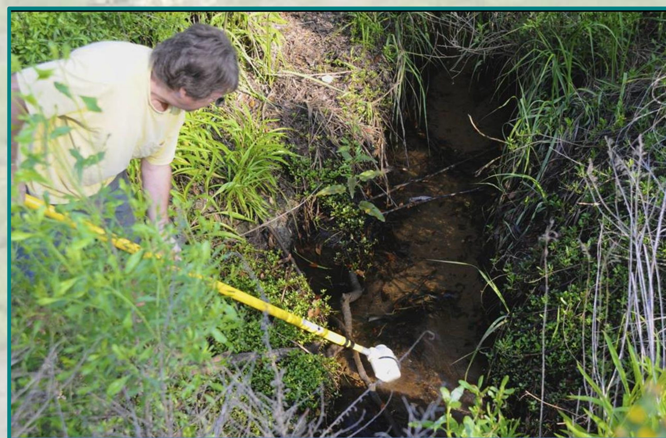
Figure 1. Volunteer Monitor collecting a water sample from tributary discharging into a tidal creek.
