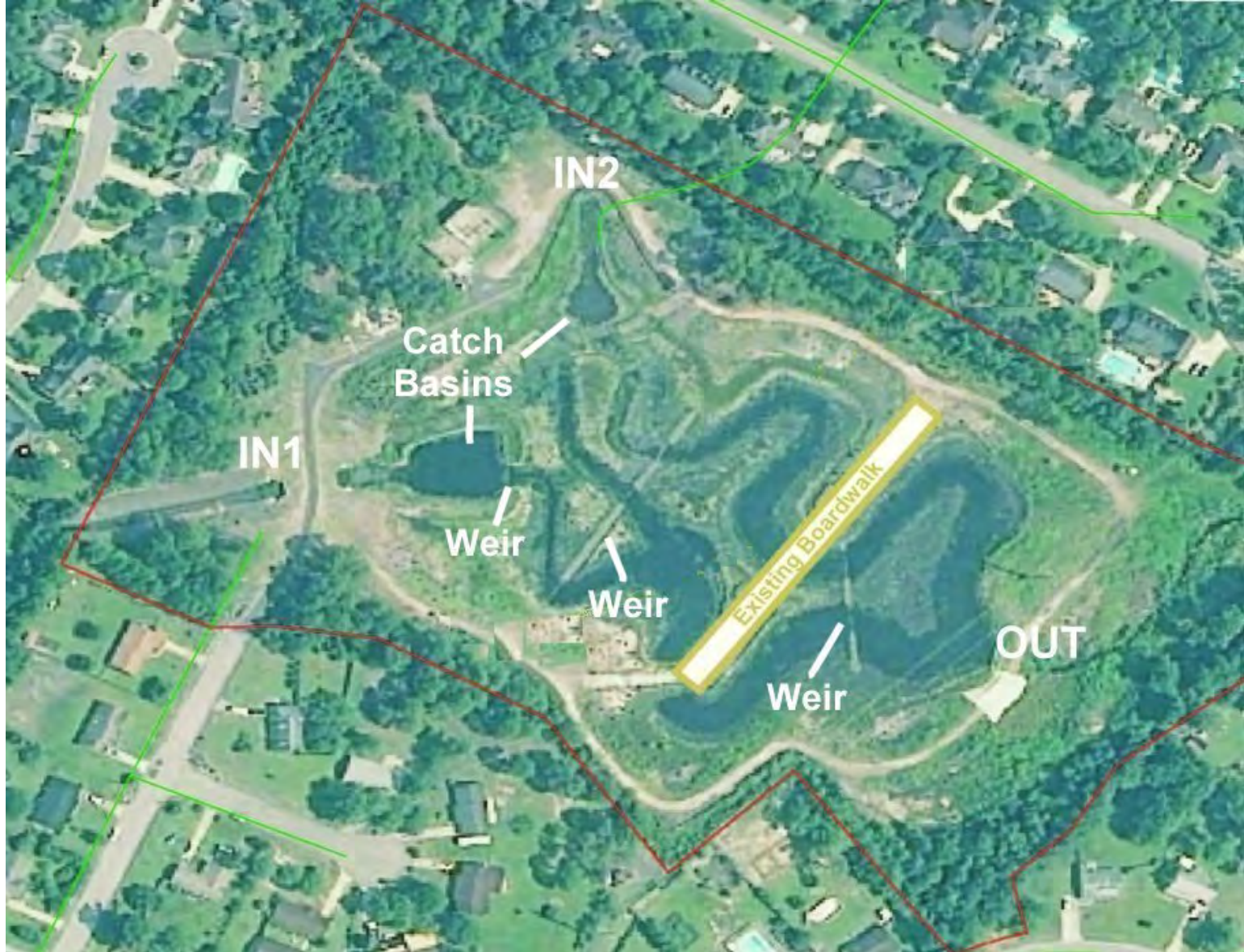
Overview of the JEL Wade constructed wetland in Wilmington, NC. It drains 589 acres (238 ha) and includes 7.6 acres (3.0 ha) of wetland and open water. Designed to treat first inch of rainfall from watershed.
