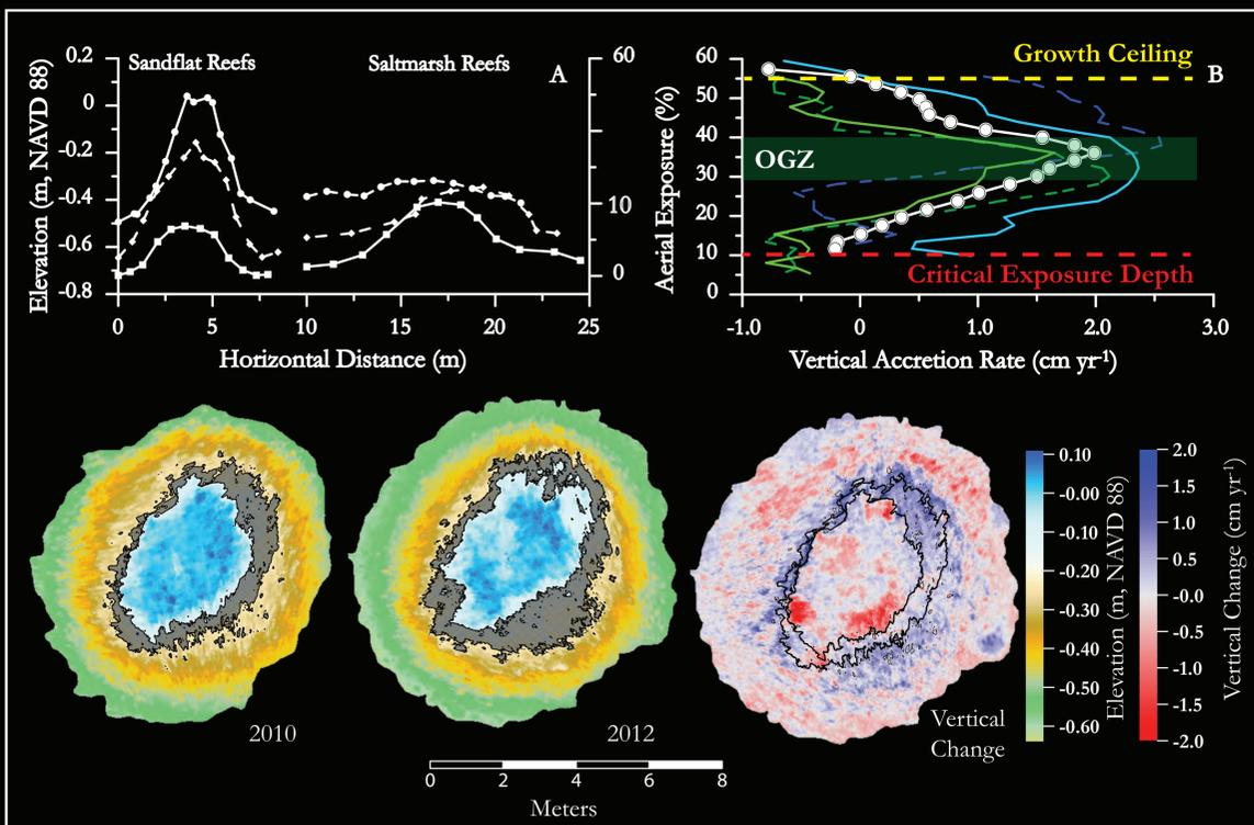
Figure 3. Oyster reef profiles by landscape and reef growth by % aerial exposure captured through laser scanning. Optimal Growth Zone (OGZ) is shaded on reef scans.
