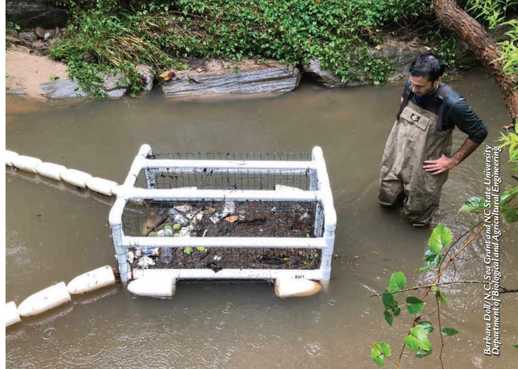
USING PVC PIPES, BUOYS, AND WIRE FENCING, RESEARCH ASSOCIATE JACK KURKI-FOX ASSEMBLED A DEBRIS COLLECTOR BASED, WITH PERMISSION, ON A DEVICE CALLED THE LITTER GITTER, PATENTED BY OSPREY INITIATIVE, AN ENVIRONMENTAL CONTRACTOR.
