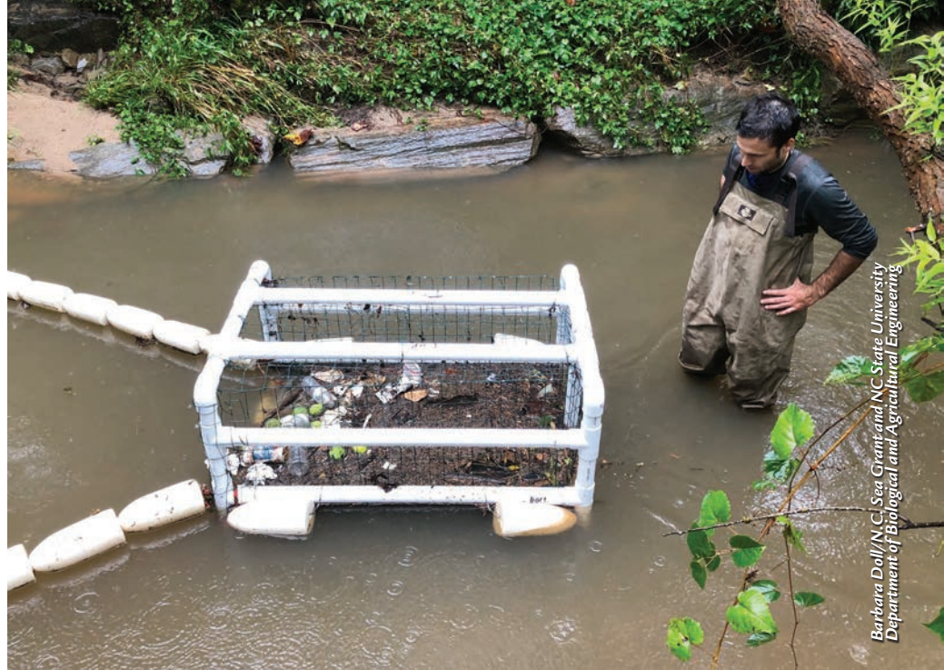
USING PVC PIPES, BUOYS, AND WIRE FENCING, RESEARCH ASSOCIATE JACK KURKI-FOX ASSEMBLED A DEBRIS COLLECTOR BASED, WITH PERMISSION, ON A DEVICE CALLED THE LITTER GITTER, PATENTED BY OSPREY INITIATIVE, AN ENVIRONMENTAL CONTRACTOR.
