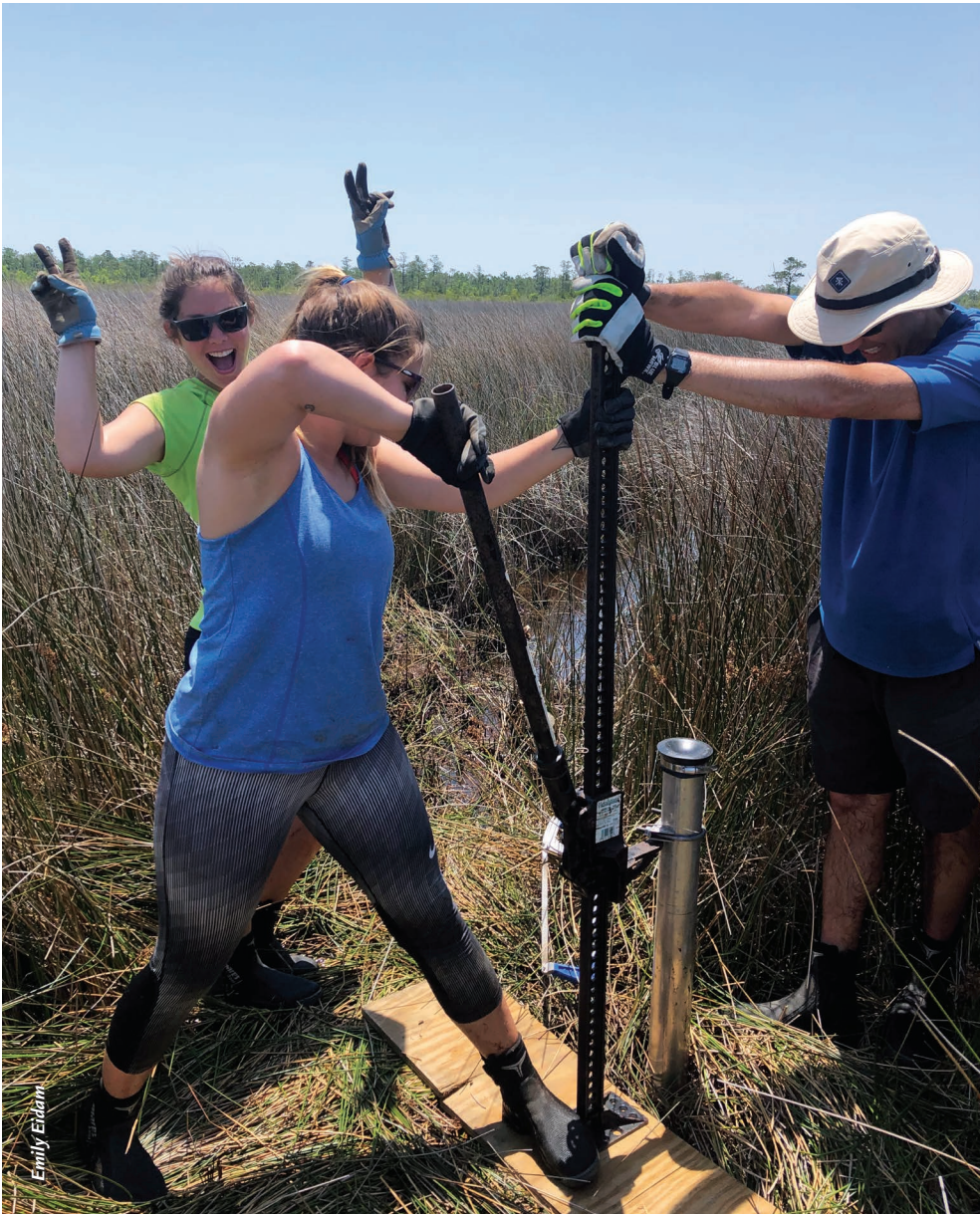
CARSON MILLER AND ANTONIO RODRIGUEZ PULL A CORE OUT OF THE SALT MARSH WITH A RATCHET JACK. IN THE BACKGROUND, MOLLY BOST OFFERS ENCOURAGEMENT.
