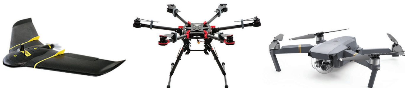
The researchers used a fixed wing drone called the eBee Plus (left), equipped with a Sensor Optimized for Drone Applications sensor. They used two rotary wing drones: the DJI S900 hexacopter (middle), equipped with a Sony 6000a digital camera, and the DJI Mavic Pro, equipped with a 12-inch megapixel CMOS camera.
