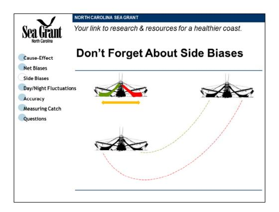
Another good reason for periodically switching the nets from side-to-side relates to the physics of turns made while towing. Water resistance and small turning radius reduces the speed of the inner net.
