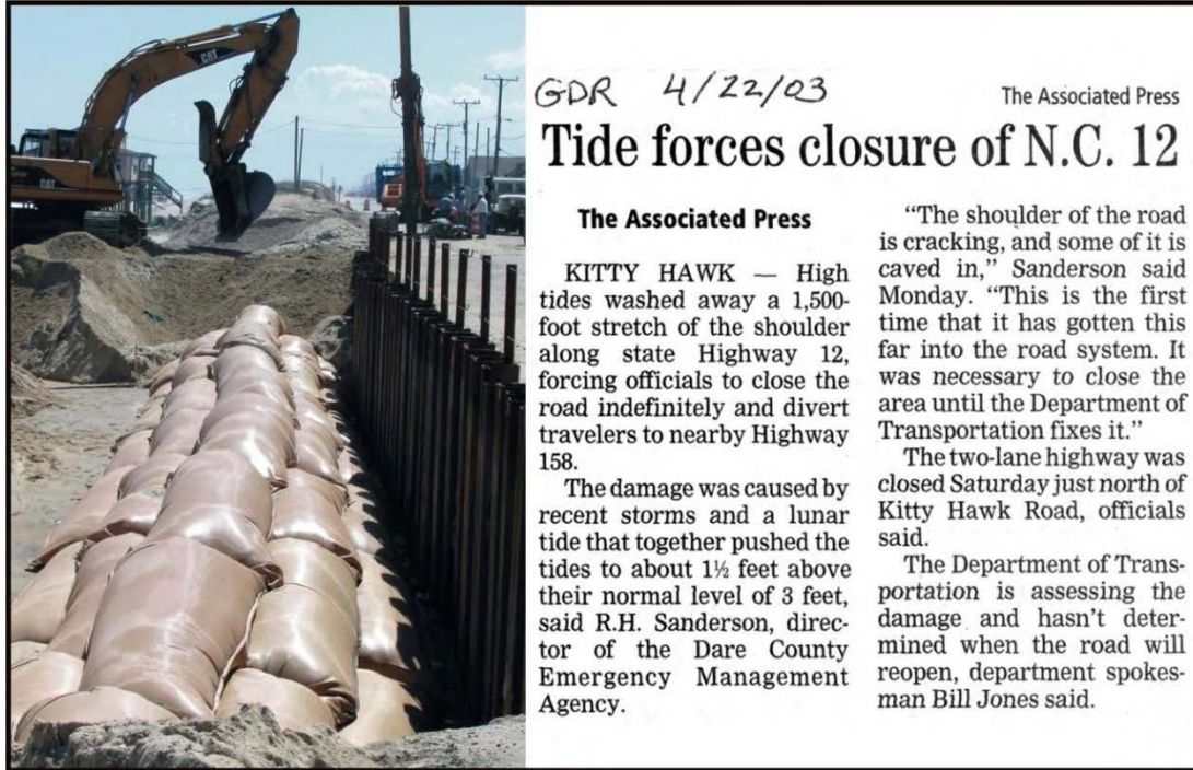
Figure 1-35. A newspaper article documents damage to N.C. Hwy. 12 in Kitty Hawk with nothing more than an abnormally high spring tide, not a storm. This segment of beach has already lost the ocean front homes and is now working on the road, which has been repaired and rebuilt many times in the last decade. The photograph was taken on March 30, 2003 and the date of the newspaper article was April 22, 2003. Photograph is by S. Riggs. Article is used with permission of The Daily Reflector , Greenville, N.C.
