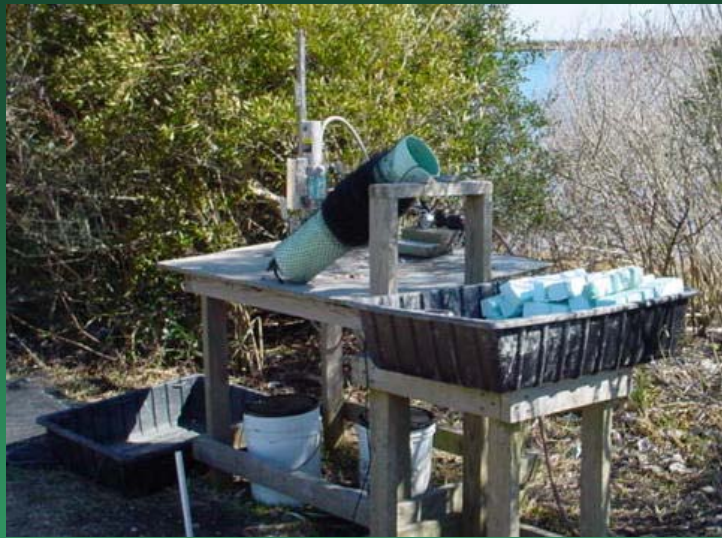
Figure 17: The clipper machine assembly line can be built with wood and plastic products. Although a clipper machine speeds up the process, the same process can be performed with hog rings.
