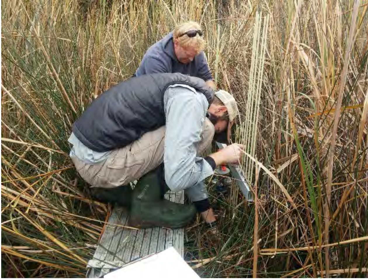
Research Staff from the N.C. Coastal Reserve use a SET at a reserve site to measure changes in the marsh's surface elevation.
