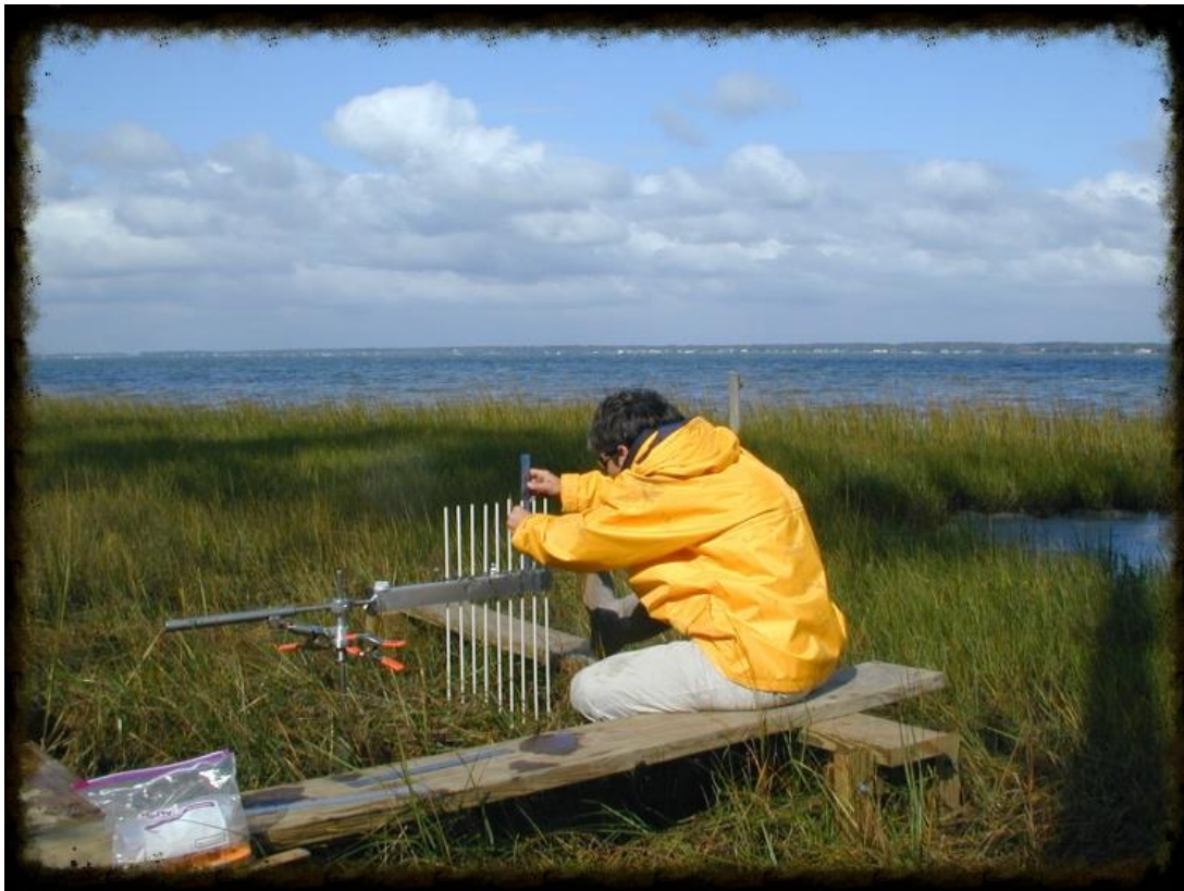
Researcher using Surface Elevation Table to monitor elevation changes in a North Carolina salt marsh.
