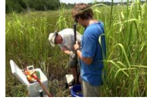
NOAA NOS staff installing a SET in the natural marsh area in Wilson Bay.
