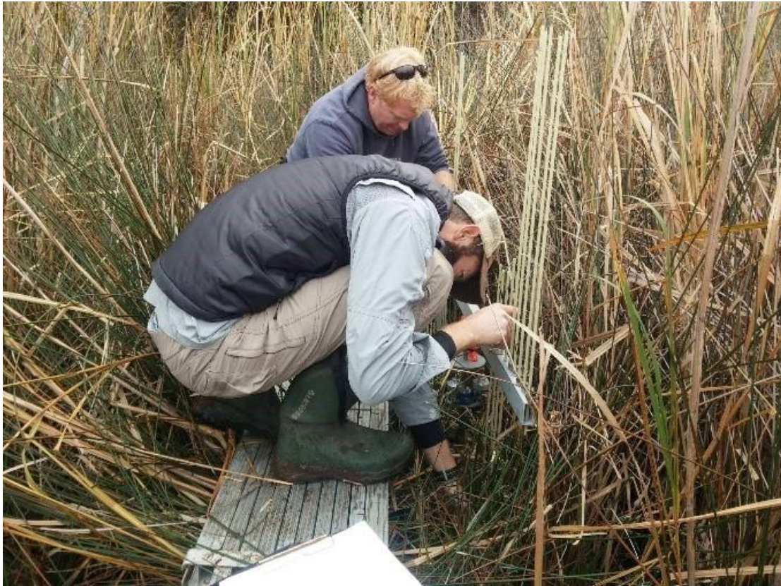
Research staff from the North Carolina Coastal Reserve use a SET at a reserve site to measure changes in the marsh's surface elevation.
